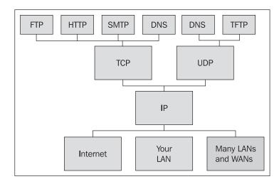
You have applications that need to reliably transfer data like FTP, HTTP, SMTP, and the zone transfers in DNS that use the TCP protocol, as well as applications that need to use a simpler protocol like TFTP and DNS requests using UDP.
