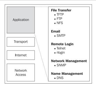
The application layer in the TCP/IP model includes protocols like FTP, SMTP, etc., with all their issues regarding data representation and dialog control. The application layer ensures that the data is properly packaged before it is passed to the transport layer.
